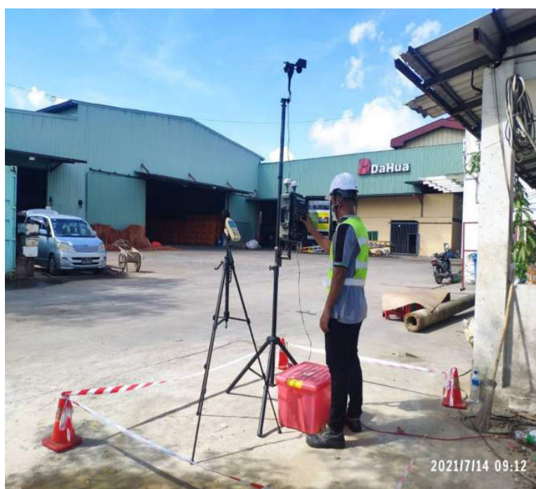
Figure 5.16 – Noise Level Monitoring
