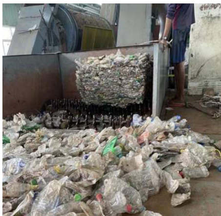
Figure – De-baling in Bale Breaker
