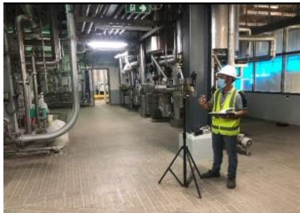
Figure 4-39 Photo of ambient air quality (PM 10 ,PM 2.5 ) and noise level (dBA) at brewing (down)
