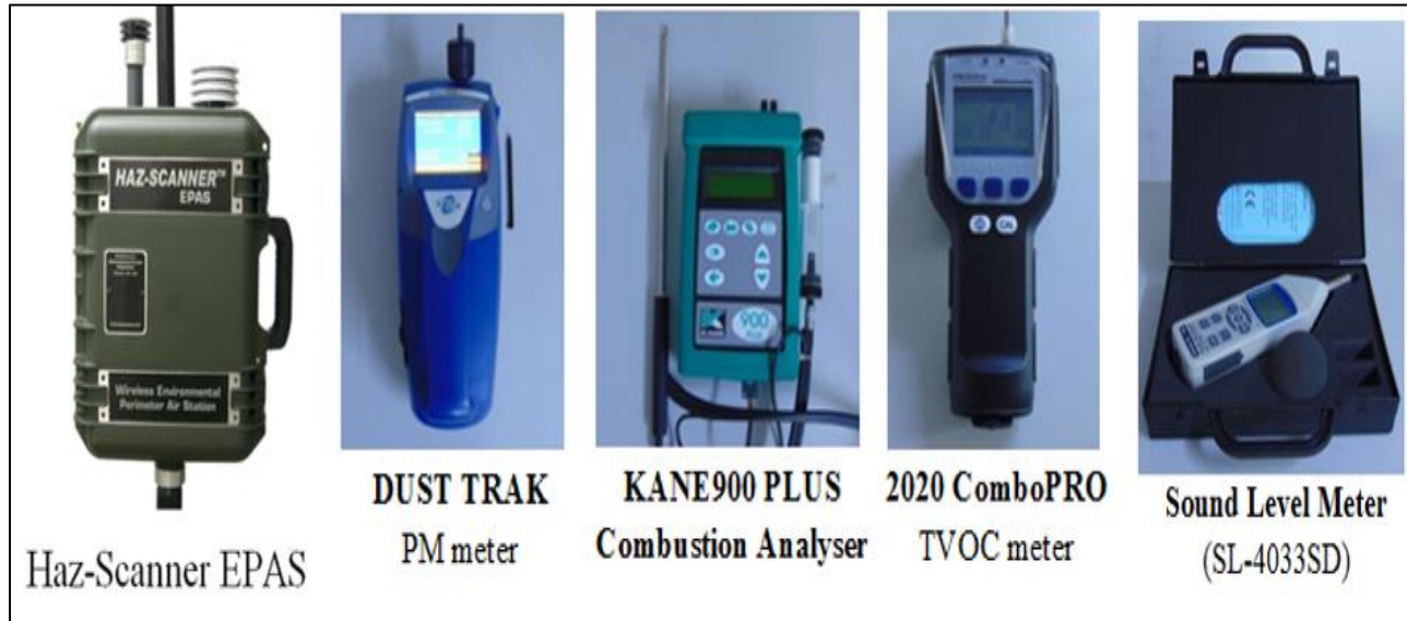
Figure 4-27 Equipments Used for Surveying the Environmental BaseLine Data
