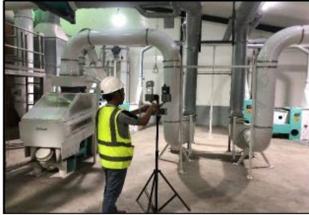
Figure 4-40 Photo of ambient air quality (PM 10 ,PM 2.5 ) and noise level (dBA) at malt milling area (up)
