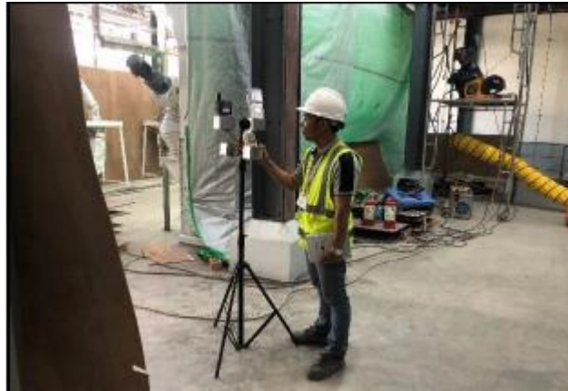
Figure 4-41 Photo of ambient air quality (PM 10 ,PM 2.5 ) and noise level (dBA) at malt milling area (down)
