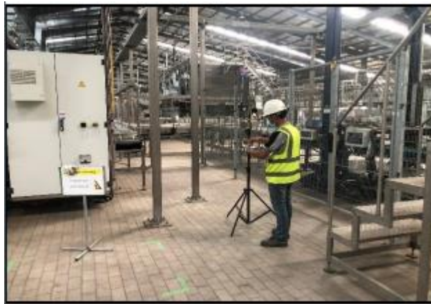
Figure 4-36 Photo of ambient air quality (PM 10 ,PM 2.5 ) and noise level (dBA) at Filling area (end point)
