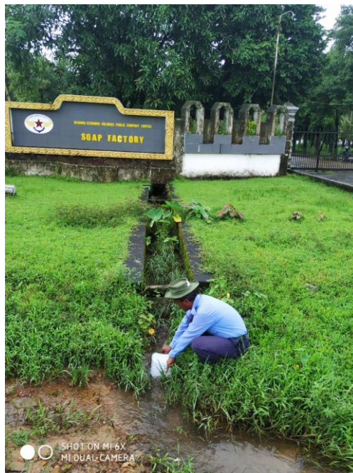
Figure 5.24 Drainage Water and Final Treated Water Samples Collection
