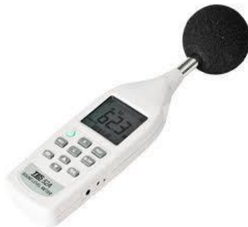
Figure 25. Noise Level Meter for Measuring Noise Level
