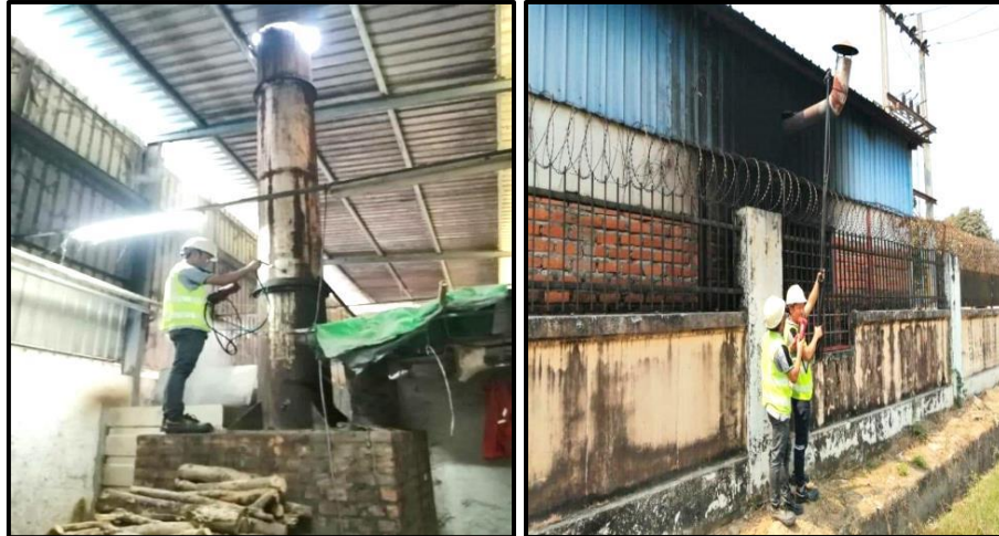
Figure 4-6 Boiler Stack Emission Measuring
