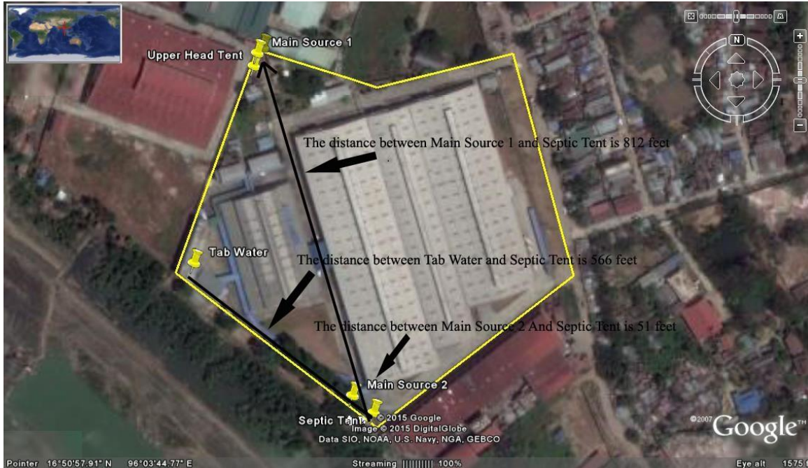
Figure 8.15 :The potable water sources, septic tank and the waste water drainage system of the factory
