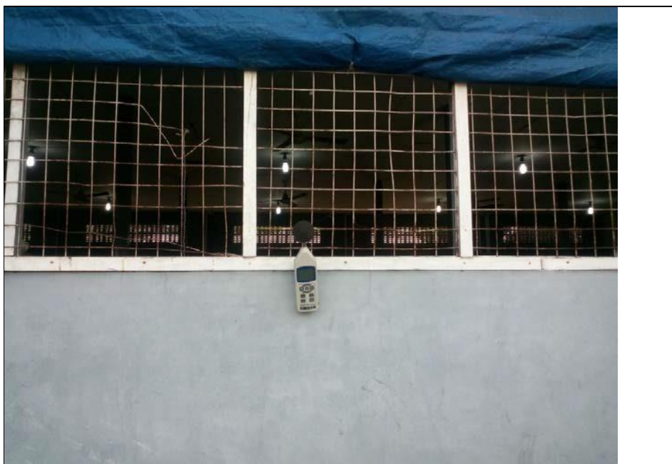
Figure 5.16: Noise monitoring at green bean sizing area of Lluvia factory
