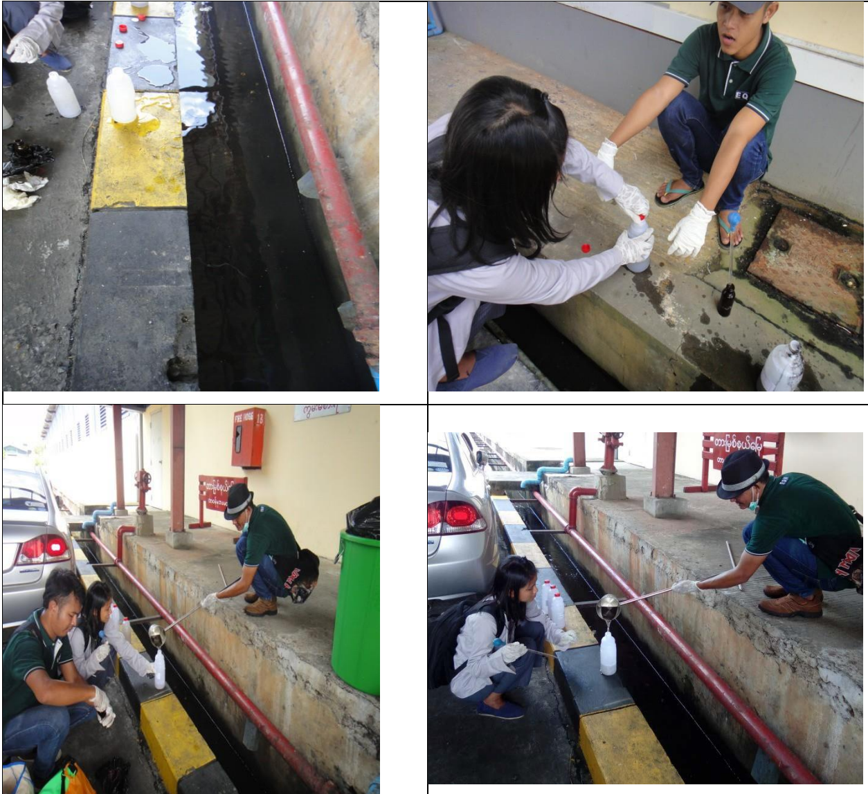
Figure 5.28: Wastewater sample collection from drainage area 1
