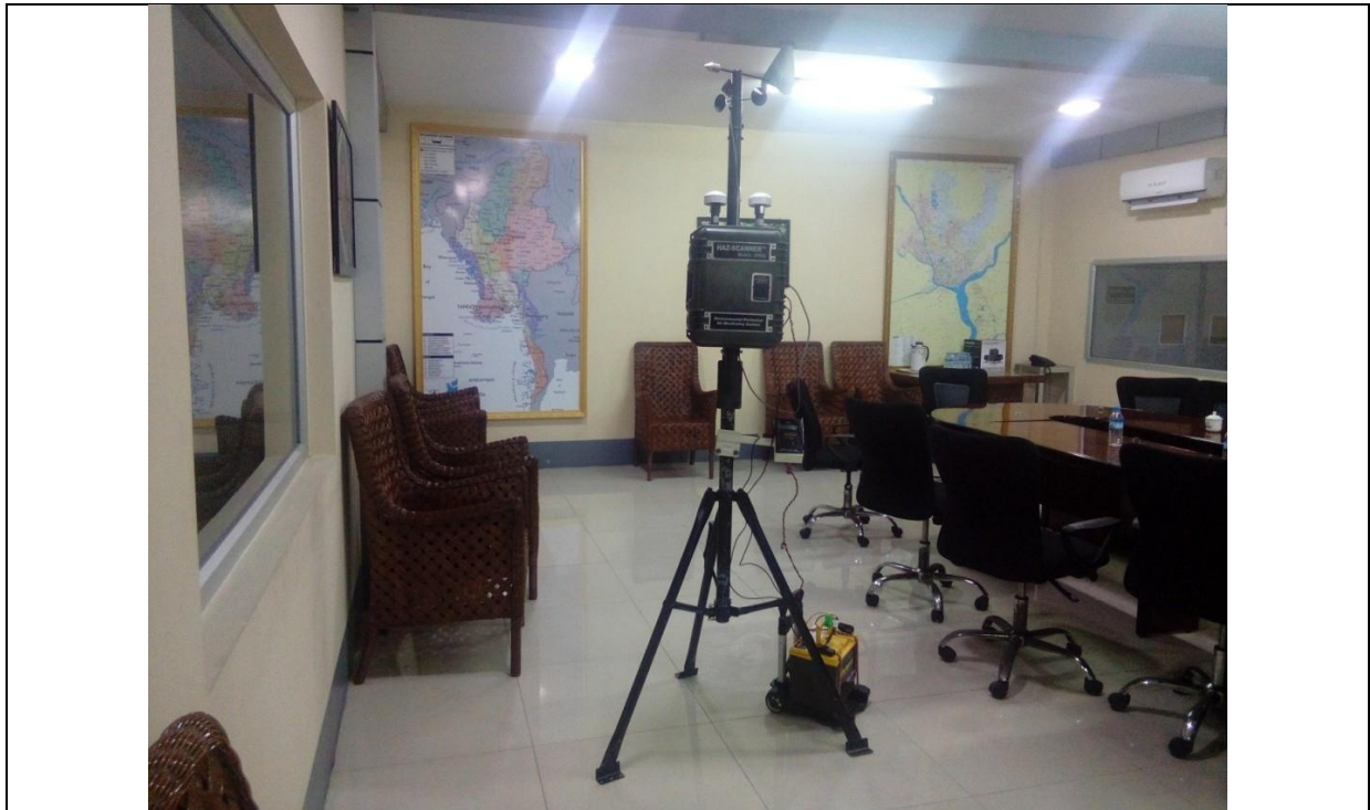
Figure 5.12: Indoor air monitoring in the meeting room (Location-2)
