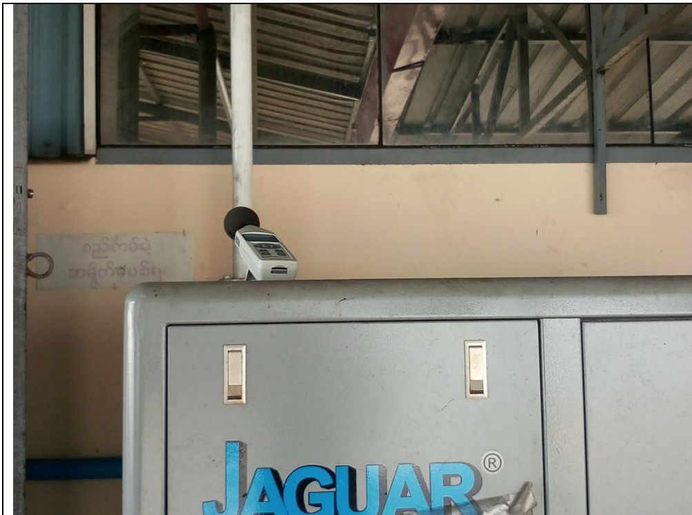
Figure 8.10: Noise data monitoring with noise meter
