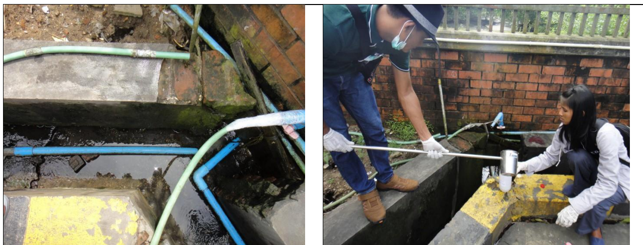
Figure 5.30: Wastewater sample collection from the final effluent pipe lines
