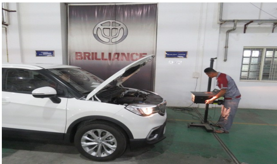
Figure – 19: Light inspection
