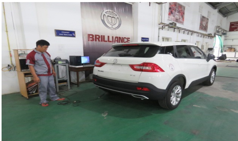
Figure – 18: Exhaust inspection
