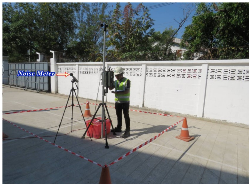
Figure-41: Measuring noise level
