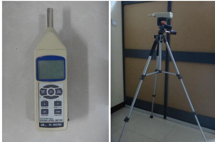
Figure 4-17 Lutron Sound Level Meter (Model - SL-4023SD)
