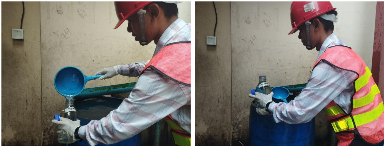
Figure 4-8 Ground Water Sampling
