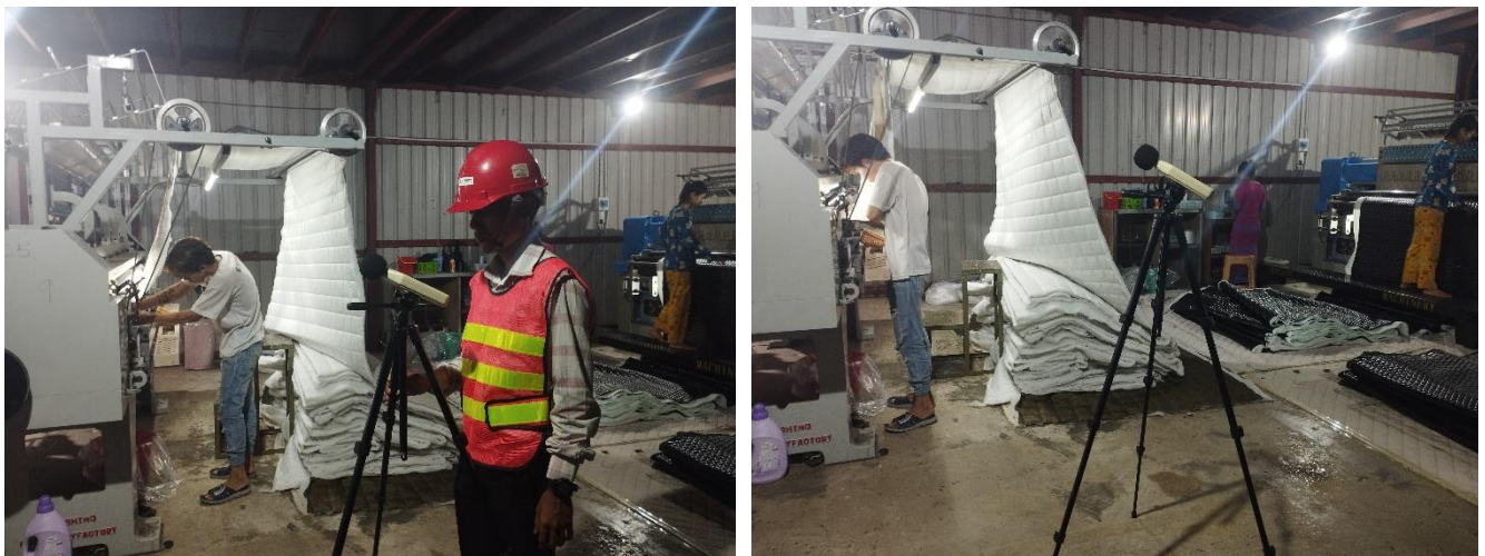
Figure 4-3 Sound Level Measurement Photo
