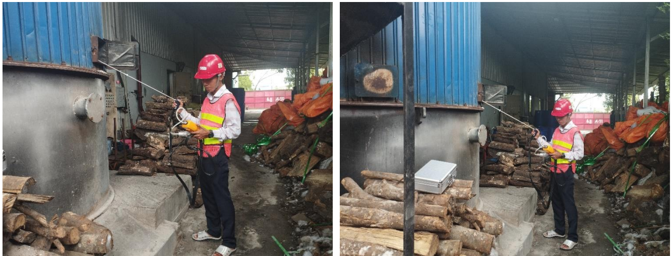
Figure 4-7 Boiler Stack Emission Monitoring
