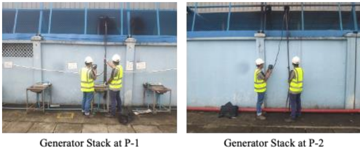
Figure 4.14 Stack Gas Emission Measurement
