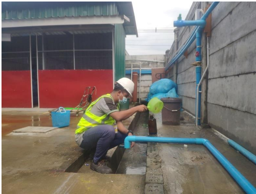
Figure 4.25 Collection of Drain Water Sample
