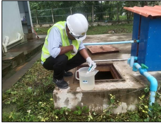
Ground Water Sampling
