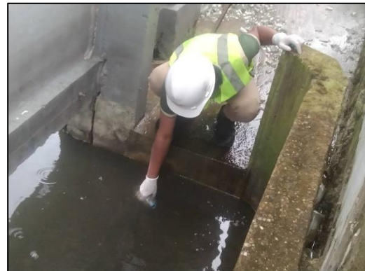
Wastewater Sampling at Final Discharge
