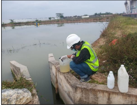
Process Wastewater Sampling
