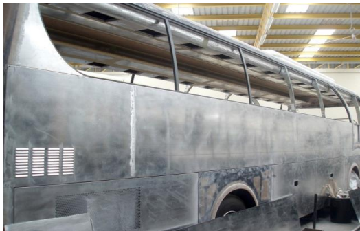
Exterior panels are mounted
