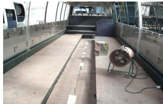
Interior fittings such as flooring, ceiling works, seats audio/video accessories are installed
