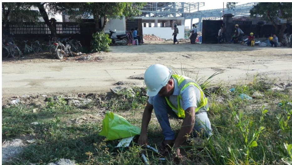
Figure 4.10 Photo of Soil Sampling
