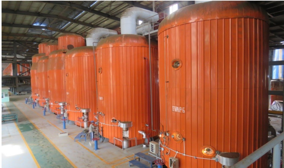
Figure-61: Boiling syrup by evaporators
