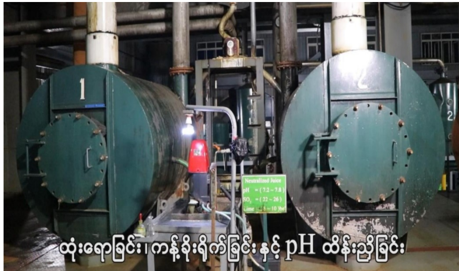
Figure-58: Mixing lime, sulphitation and regulating pH
