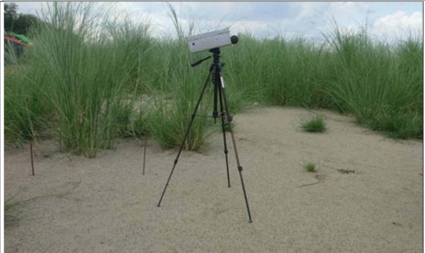
Figure 5.10 Noise monitoring station at the project compound
