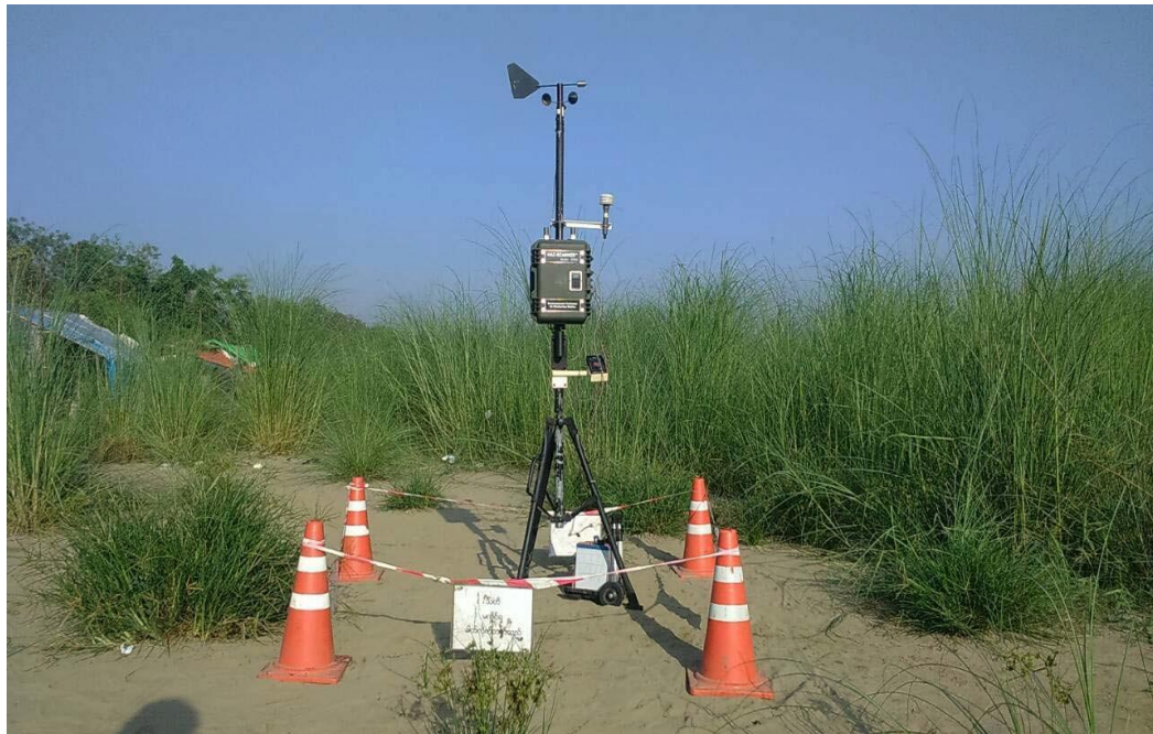
Figure 5.5 Ambient air monitoring at the project compound (Location-4)
