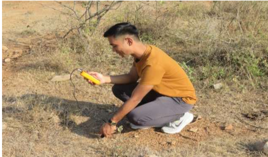
Figure-35: Measuring vibration level at project site
