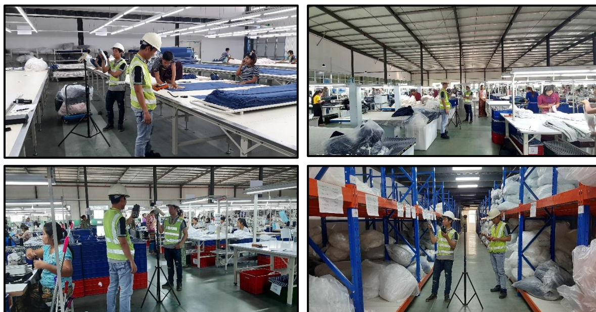
Figure 4-5 Air Quality, Noise and Light Meter Measuring
