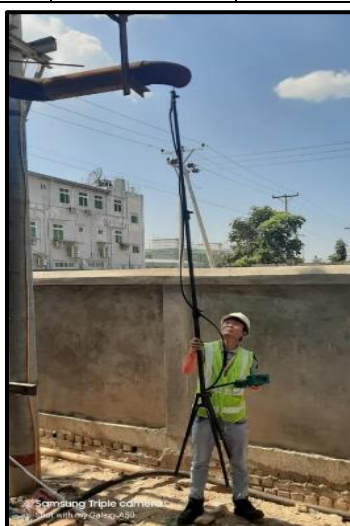
Figure 4-6 Generator Stack Emission Measuring
