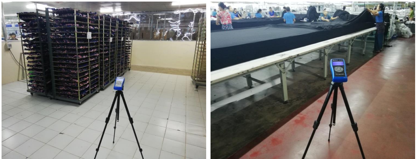
Figure 4-1 Air quality measurement at the project site
