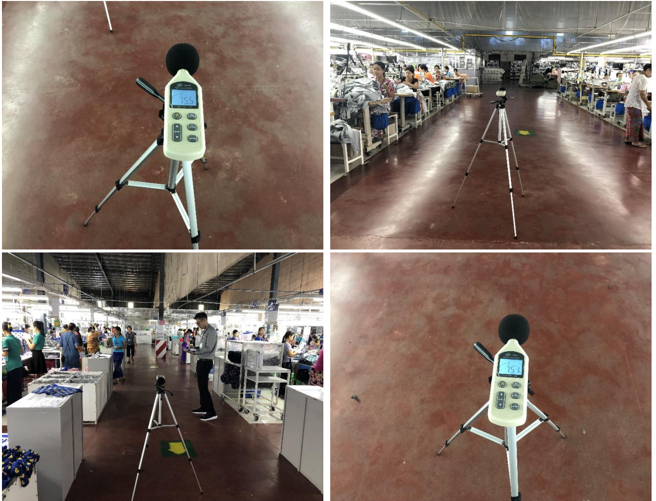
Figure 4-5 Noise level measurement in the factory
