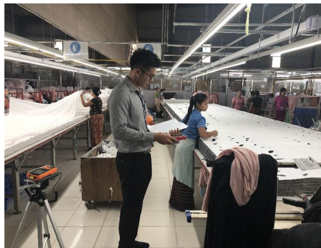
Light measure at cutting line
