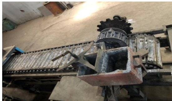
Figure 3.36 Casting into Lead Ingots
