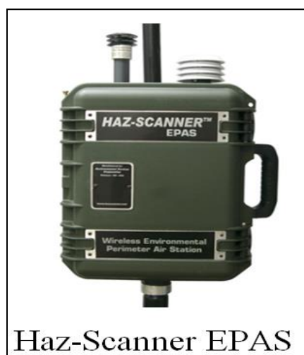
Figure 4.10 Ambient Air Quality Measuring Equipment (Haz-Scanner)
