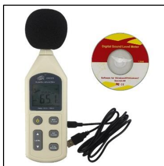
Figure 4.13 Sound Level Measuring Equipment (Sound Level Meter)
