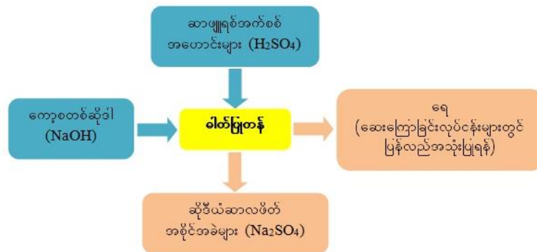
Figure 3 Neutralization Process for Spent Electrolyte
