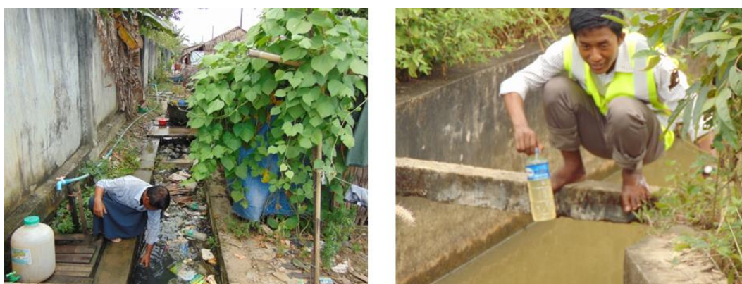
Figure 4.23 Taking Wastewater Samples from Municipal Sewage in front of Project Site and Zone during Construction Phase
