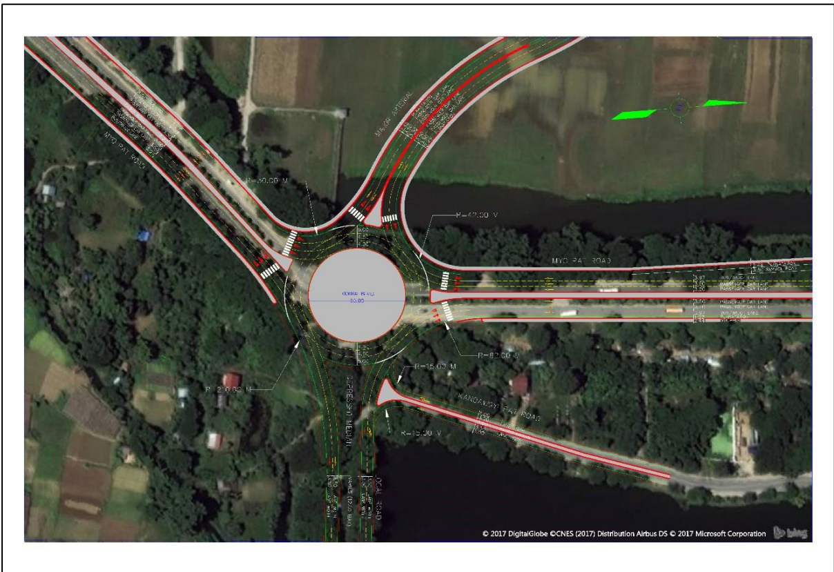
Figure 3-29 At-Grade Intersection of RA2
