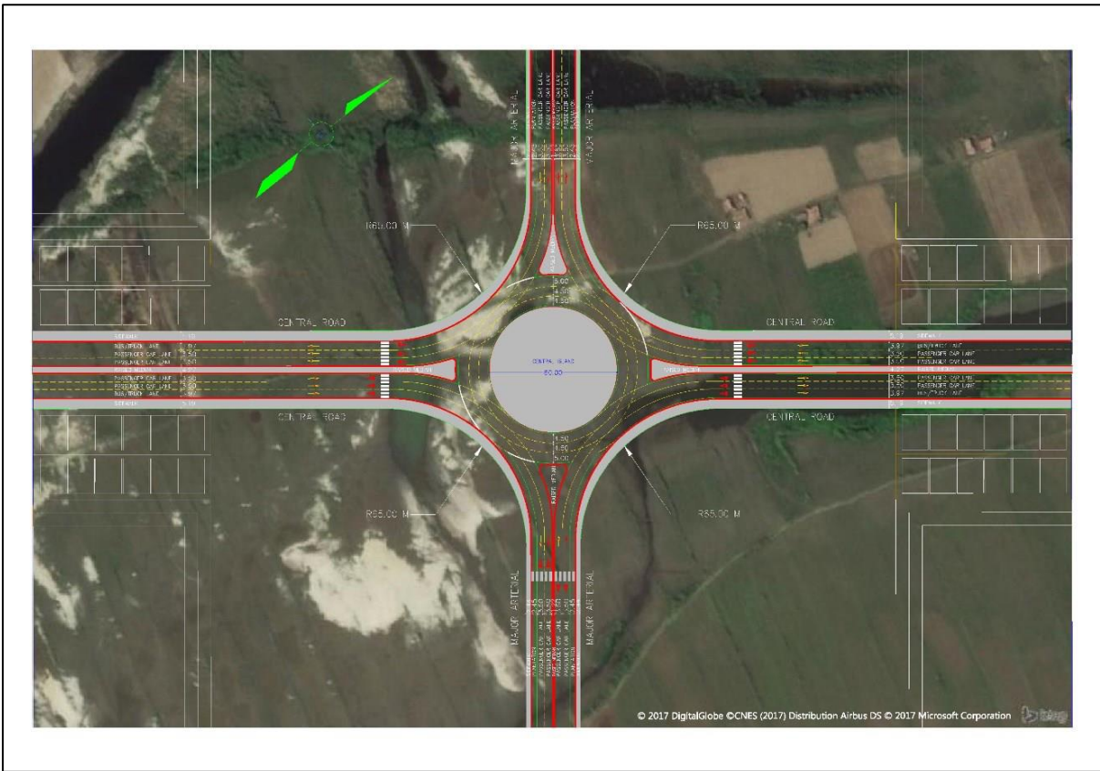
Figure 3-33 At-Grade Intersection of RA6
