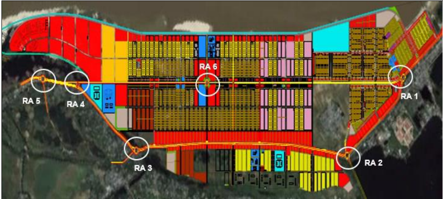
Figure 3-27 Locations of At-Grade Intersection
