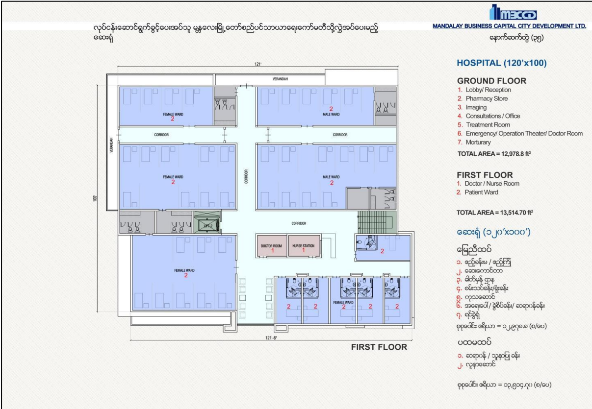
Figure 3-52 First floor plan of the hospital
