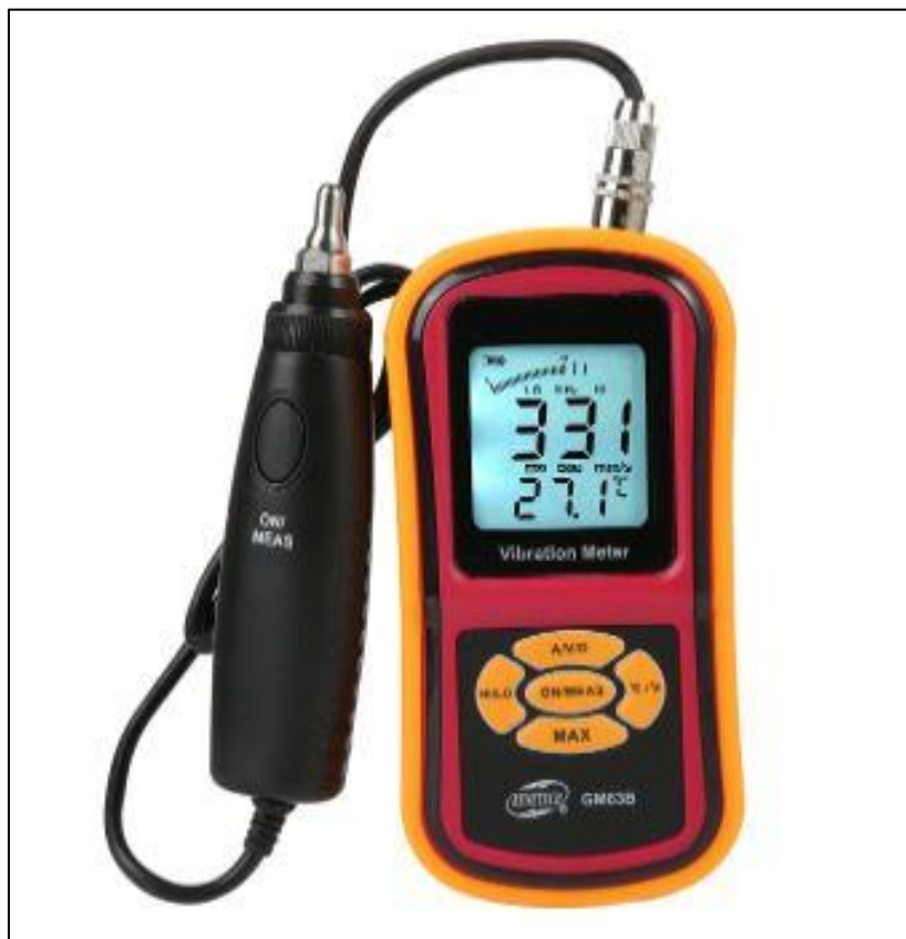
Figure 4-112 BENETECH Vibration Monitoring Equipment
