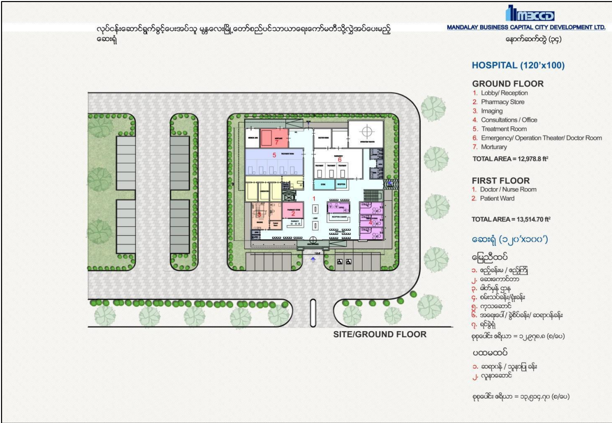
Figure 3-51 Site ground floor plan of the hospital
