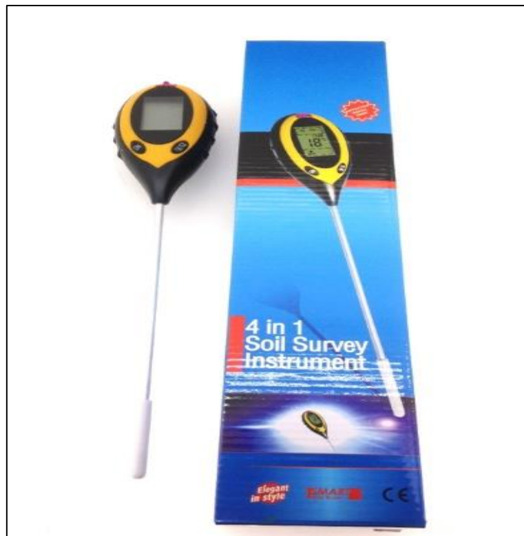
Figure 4-114 4 in 1 Soil Survey Instrument
