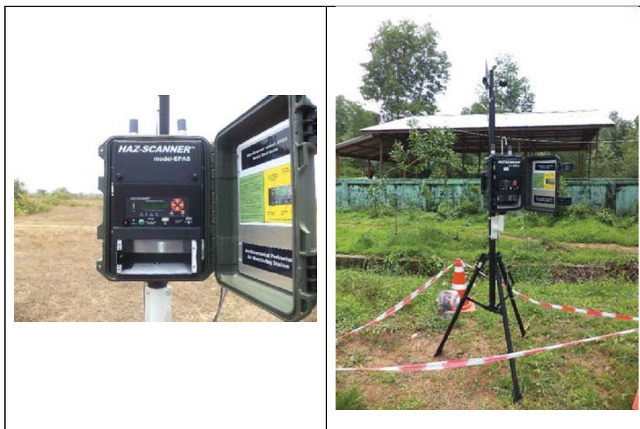
Figure 1.1-2 Haz-Scanner Environmental Perimeter Air Station
