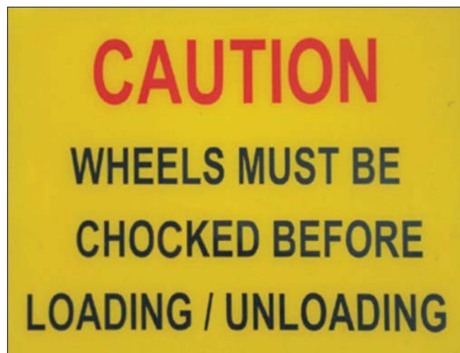
Display of cautionary signage to remind driver to provide wheel chock for their vehicle / mobile machinery
