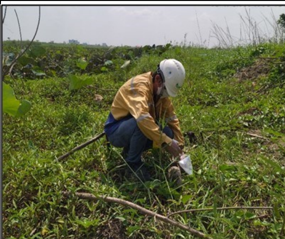
Soil Sampling at Waste Disposal Site (SP 3) Dry Season
