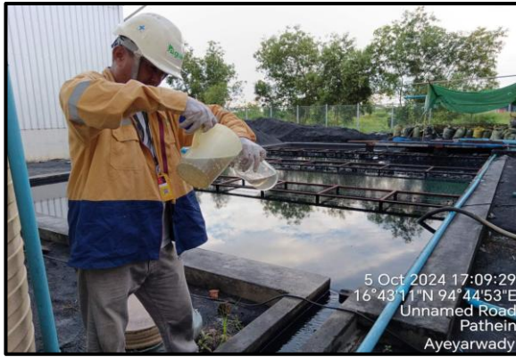
Effluent Water Quality Sampling (Point-1)
