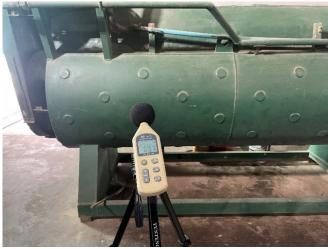
Figure 4-13 Noise Level Measurement Photo
