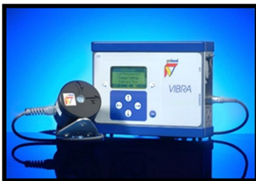
Figure 4-39 Vibrating measured instrument
