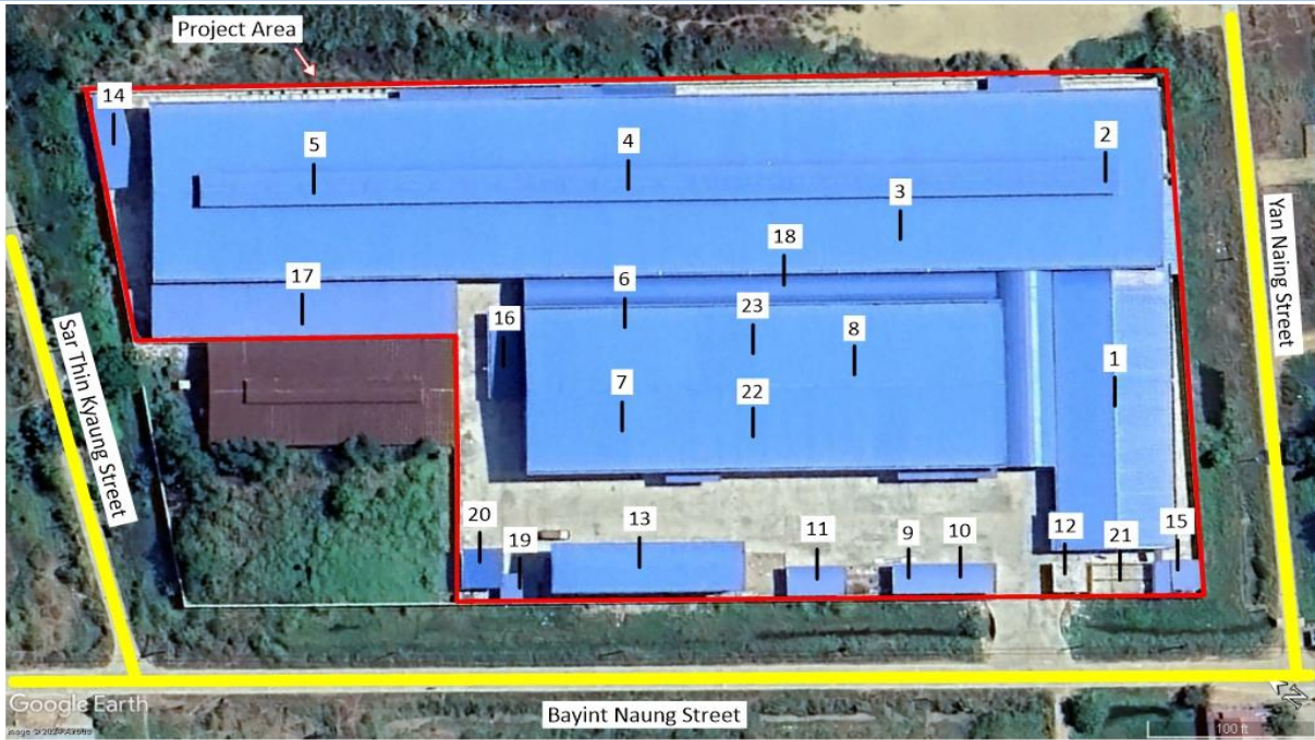
1 - Final Product Packing Storage Area, 2 - Final Product Storage Area, 3 - Packing Area, 4 - Sewing Area, 5 - Assemble Area, 6 - Printing Area, 7 - Cutting Area, 8 - Office Area, 9 - Clinic Room, 10 - Interview Room, 11 - Chemical Storage Room, 12 - Security Room, 13 - Dormitory (1), 14 - Dormitory (2), 15 - Firefighting Equipment, 16 - Waste House, 17 - Toilet, 18 - Canteen, 19 - Water Purify Room, 20 - Store Room, 21 - Generator & Transformer, 22 - Store Department, 23 - Warehouse
