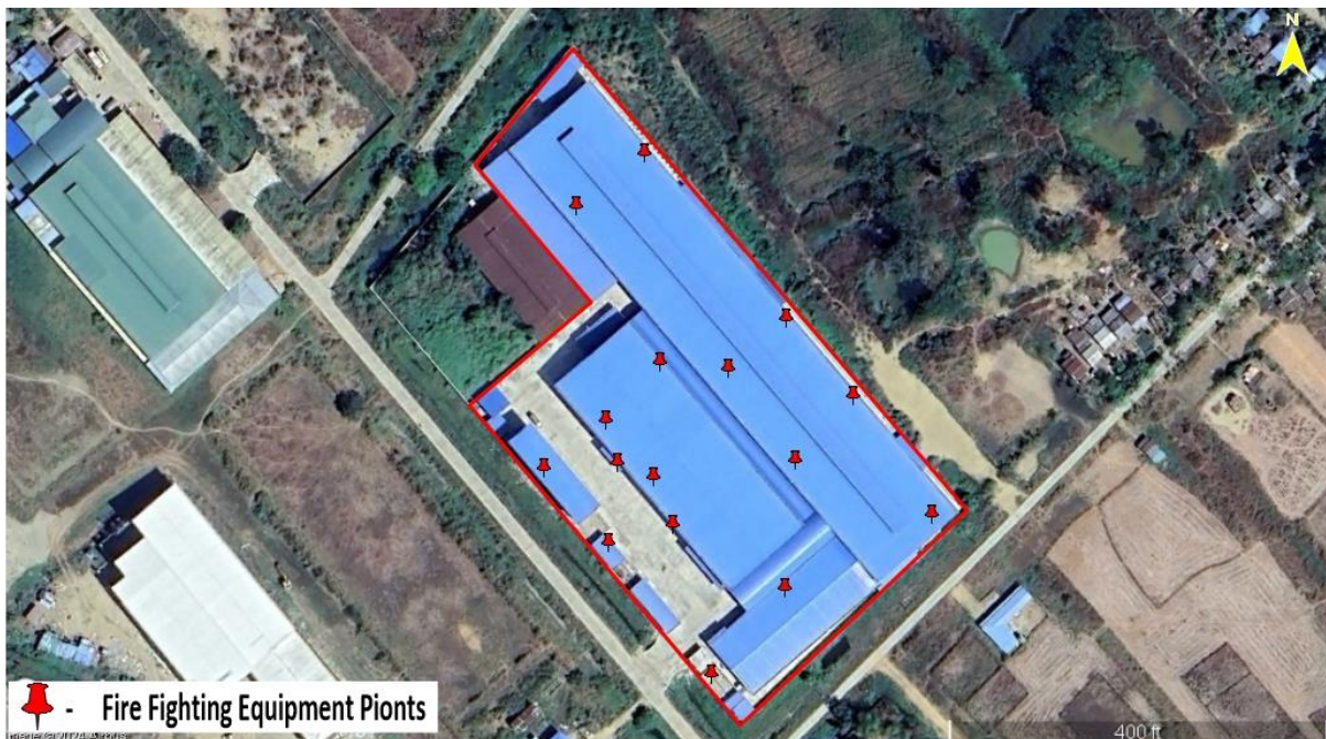
Figure 6.9 Fire Fighting Equipment Location Points
