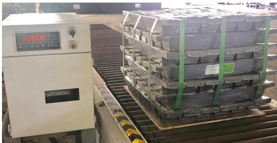
Figure 3-19 Bundle Weighting System with Printer
