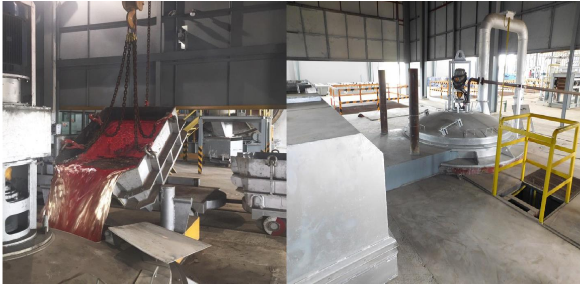
Figure 3-7 Locomotive Cart & 60 Tons Kettle
