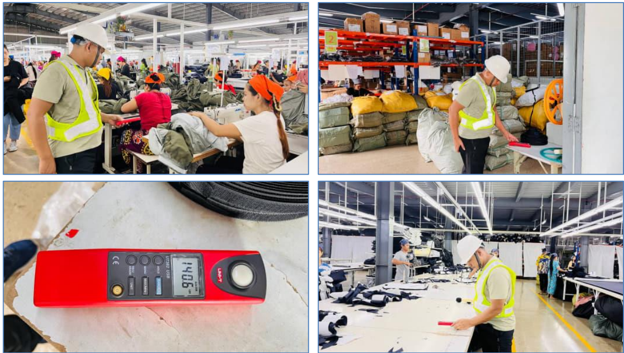
Figure 5-13 Some Record Photos for Light Measuring
