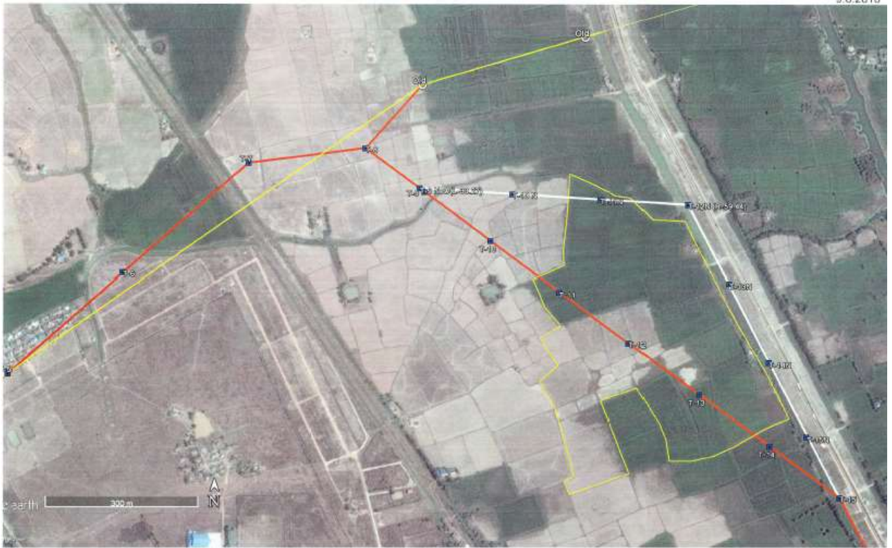
Figure 1: Proposed Tower locations near Thanlyin Sub-Station
