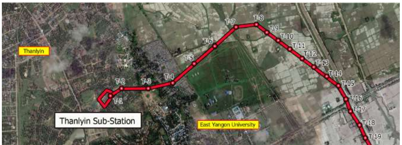
Figure 1: Proposed Tower locations near Thanlyin Sub-Station
