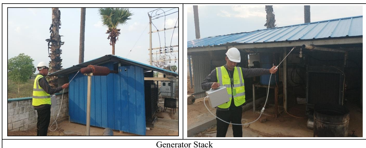
Figure 4-34 Stack Height Emission Monitoring Equipment (Oceanus OC-1000)
