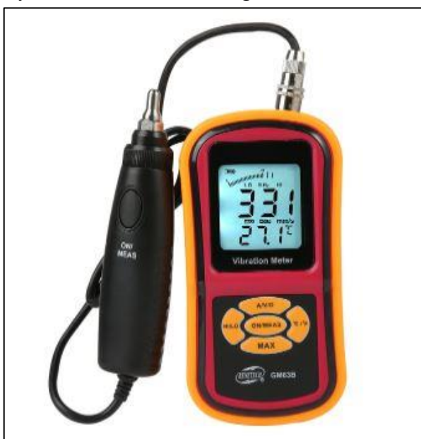
Figure 4-56 BENETECH Vibration Monitoring Equipment
