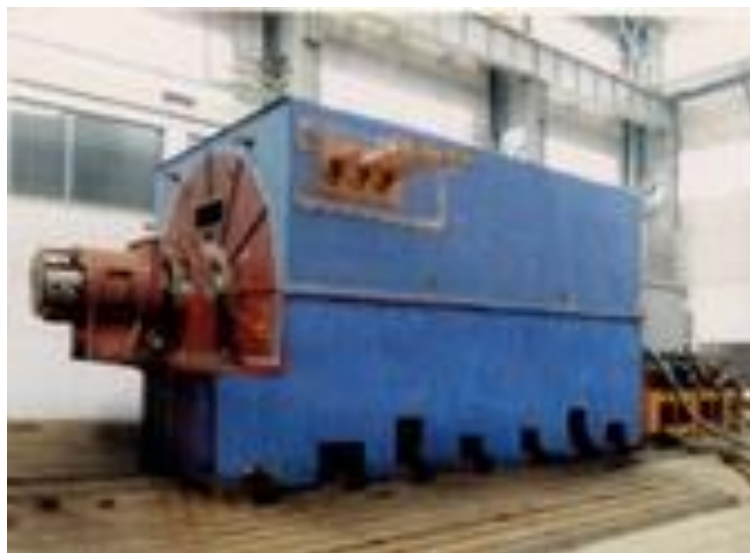
Photo 3-28: QFR-135-2Gas Turbine-Generator (Specimen)
